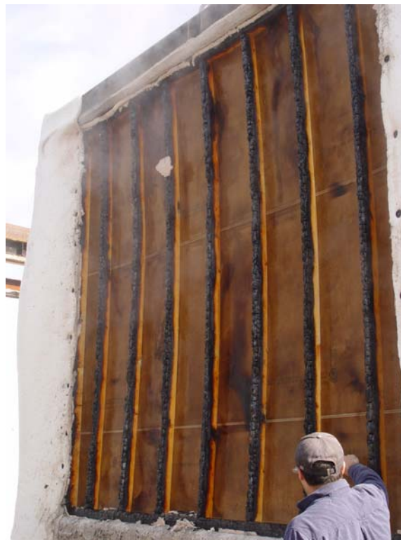
Post exposure, cavity exposed
